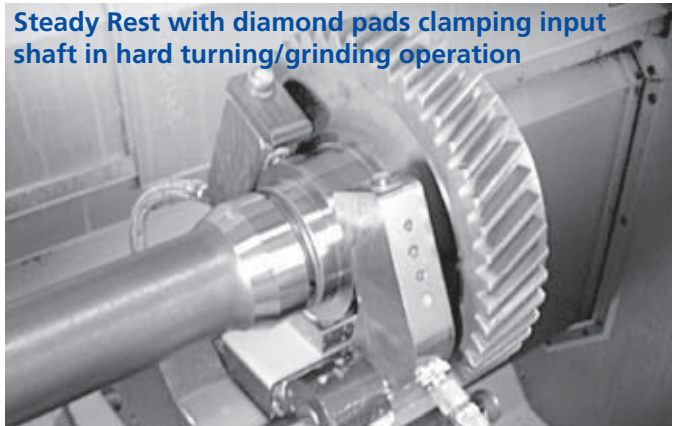
Steady Rest clamping aircraft shaft
